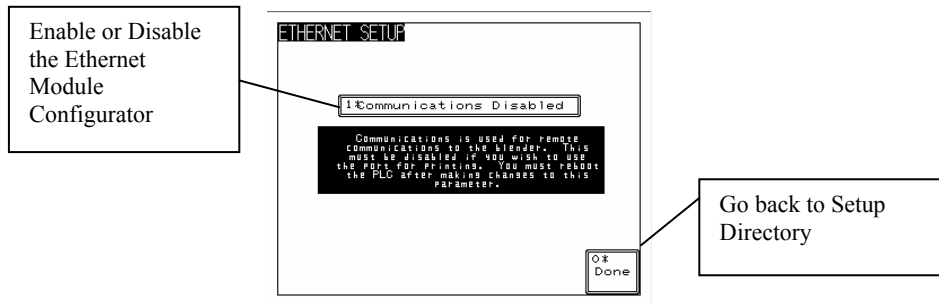
Figure 31: Ethernet Setup Screen
